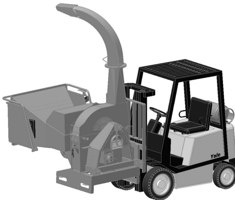
Figure 2 Lifting the machine using a forklift truck
